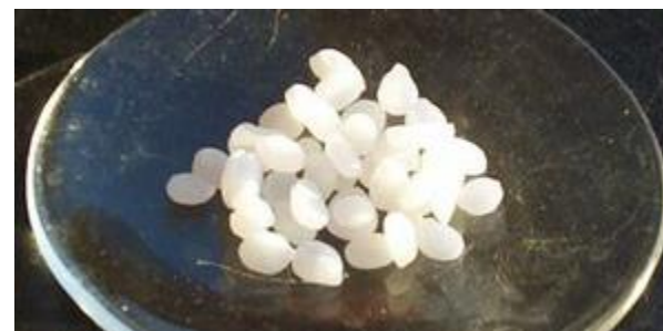
Figure 10.6: Sodium hydroxide is generally sold as pellets with about 98% purity. They quickly absorb moisture from the air, eventually forming their own solution.
